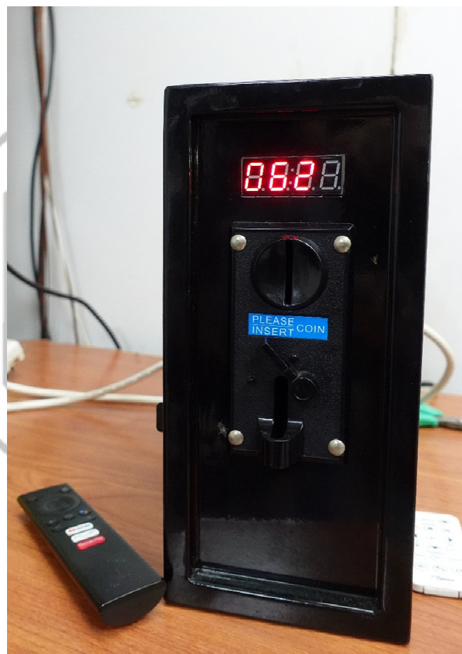
Fig. 4.2 The modified coin-operated karaoke machine connected to online application (Photo by the author)
