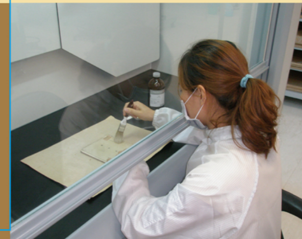
Remove dirty air with the exhaust cabinet.
